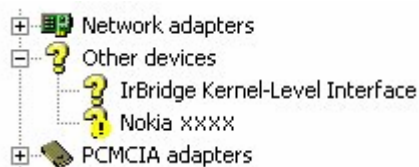
Figure 3. Unknown device (xxxx stands for the four-digit model number of your phone)
